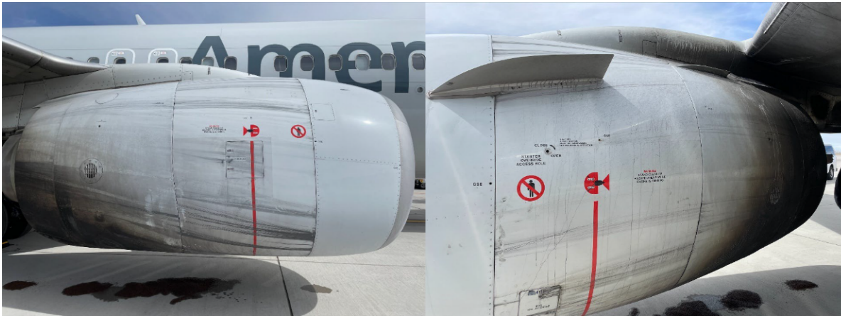
Figure 2. Photos showing the markings and damage to the right engine nacelle. The photo on the left shows the outboard view and the photo on the right shows the inboard view.
