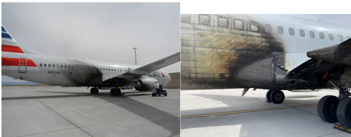
Figure 1. Photos showing the damage to the right side of the airplane.
